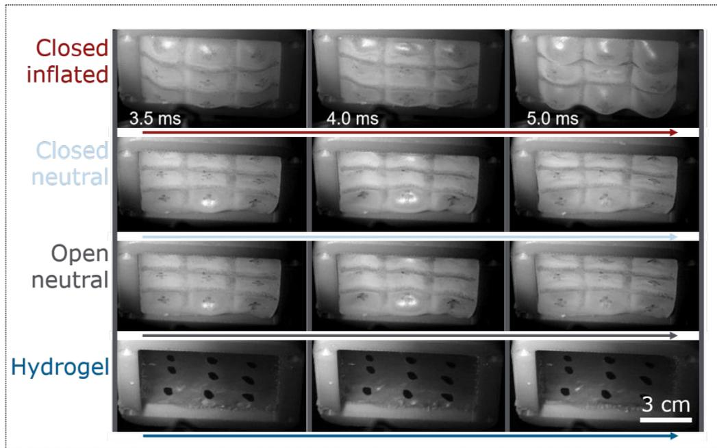
**Figure S-4.** Extended results from **Figure 7b**. The samples are blasted with 120 kPa of peak shock overpressure. The presence of air in the SRSL exhibits external deformation (rebound) whereas the hydrogel only has small internal deformations/compressions.
