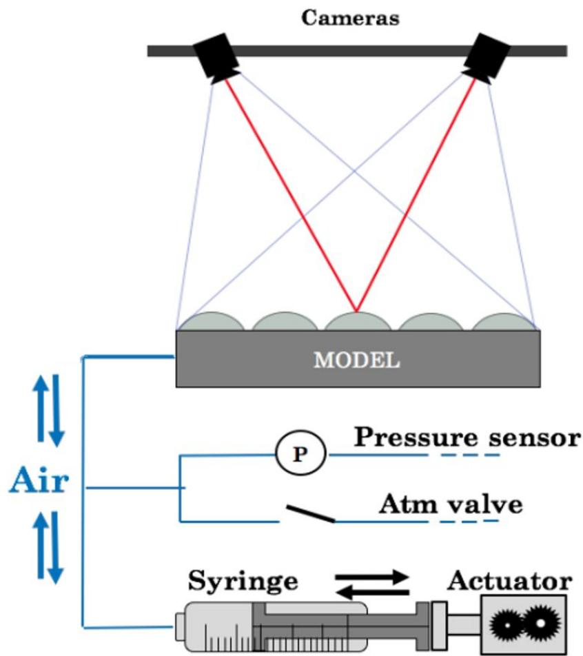
**Figure S-2.** Set up for Pressure-Volume evaluation (using CiT) and Digital Image Correlation (DIC) tests.
