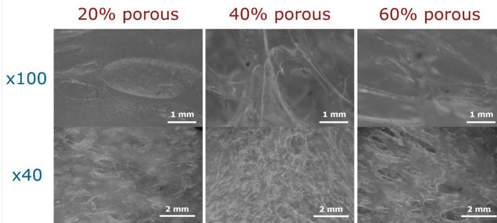
**Figure S-1.** Microscope images of porous Ecoflex 00-30 at 20%, 40% and 60% porosity. There are round pores into the material with little connectivity (pathway) and the pores become larger with increasing porosity and irregular.
