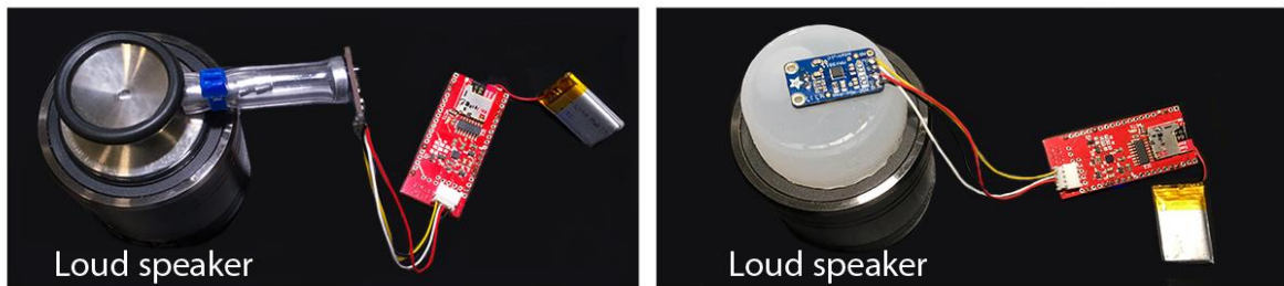
Figure S4. Re-recording of the reference heart sounds (downloaded from an online repository) using a loudspeaker. Re-recording with a (Left) commercial stethoscope; (Right) 15 mm water-silicone composite transducer.
